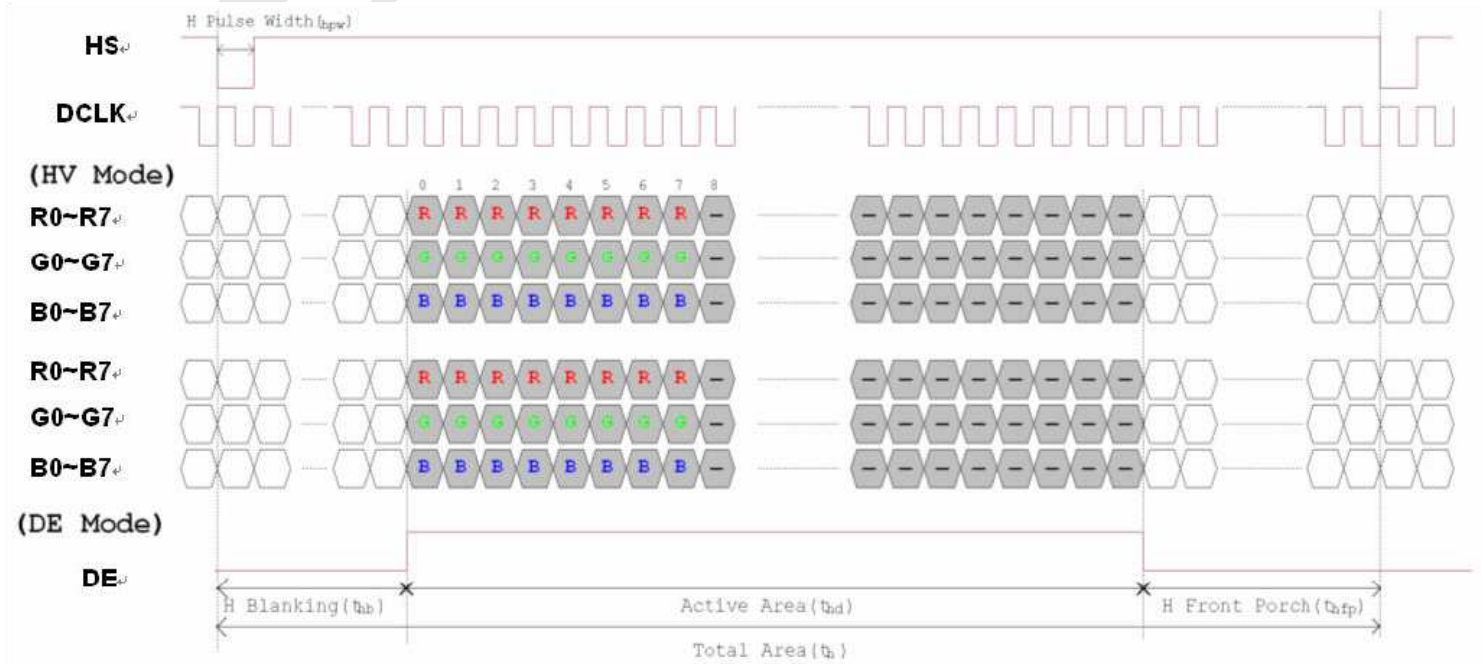
Figure 3. 1 Horizontal input timing diagram.
